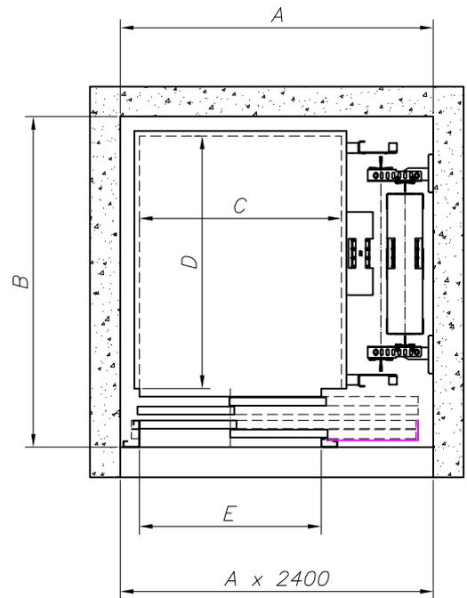
1. Deviations of the hoistway width and depth from the nominal sizes – between –20 mm +30 mm.
